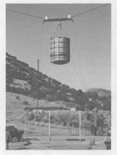
TRUPACT-II nuclear waste transportation container is readied for a drop test at Sandia's 5000-ft. aerial cable facility.
